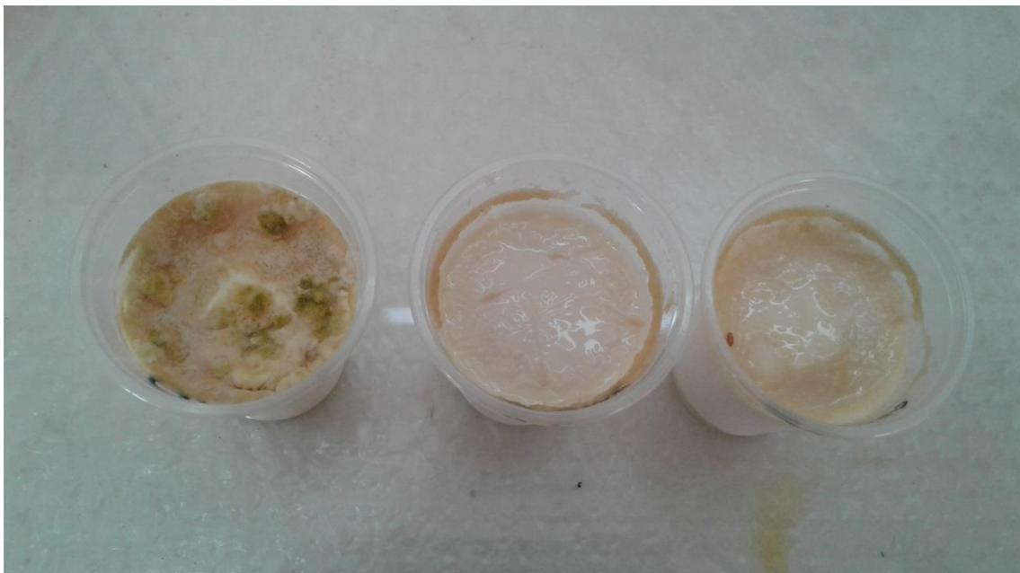
Microbial growth is found on control milk and clear milk can be seen on one time passed and three times passed milk.
