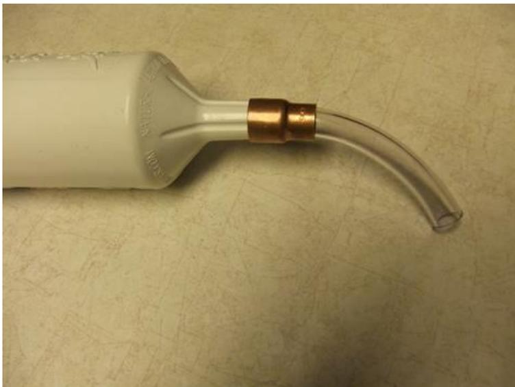
You should be able to find a copper coupling like the one in the picture above (also below) at any hardware store.
